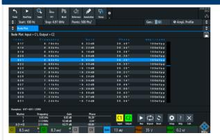
The measurement results table provides detailed information about each measured point (frequency, gain and phase shift). When using markers, the applicable row of the results table is highlighted. Screenshots and table results can be quickly saved to a USB device for reporting.
