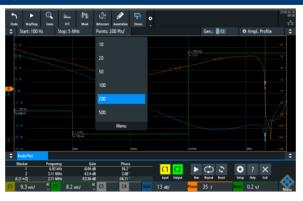
Choose the points per decade to set up and modify the resolution of your plot. The oscilloscope supports up to 500 points per decade. Drag markers to the desired position directly on the plotted trace and easily determine the phase and gain margin.
