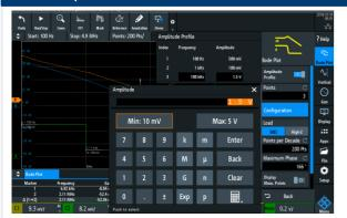
Profiling the amplitude output level of the generator helps suppress the noise behavior of your DUT when measuring the control loop response or PSRR. Profiling also improves the signal-to-noise ratio.
