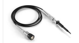
Accurate control of loop response or PSRR characterization highly depends on choosing the right probes, since the peak-to-peak amplitudes of both  $V_{\rm in}$  and  $V_{\rm out}$  can be very low at some test frequencies. The low-noise R&S\*RT-ZP1X 1:1 passive, 38 MHz bandwidth probe improves dynamic range.
