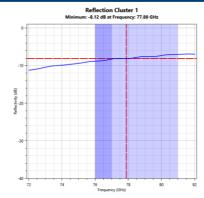
Ideally, the frequency response minimum is in the operating frequency range for the radar sensor in combination with the DUT. Shifted minimums indicate issues with the electrical thickness of the DUT, requiring thickness adaptation based on frequency responses in reflection measurements
