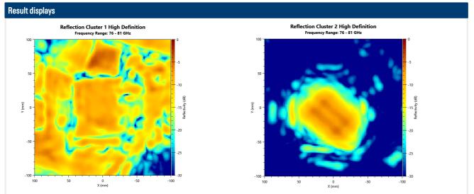
The resulting reflection image displays the measured levels in different color according to the dB level. The reflected image is evaluated and displayed separately for each cluster. The color range depends on the selected color scheme. A color map next to the image explains which levels correspond to which color.
