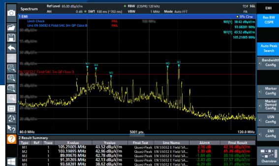
Max. peak detector-based signal sweep (top) and quasi-peak detector-based disturbance maxima analysis (bottom)
