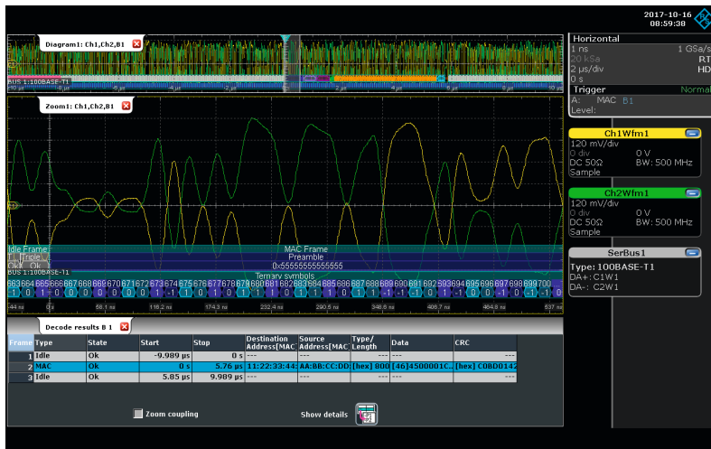
Decoding of the electrical 100BASE-T1 bus levels. The two levels of the differential 100BASE-T1 signal are clearly visible along with the decoded telegram content.
