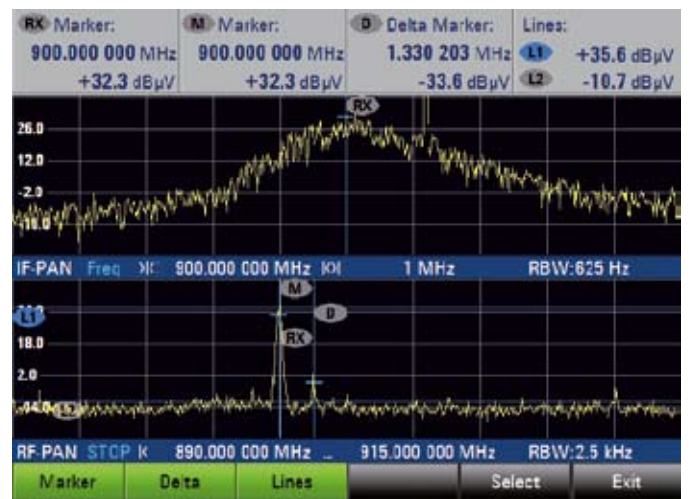
Interference from a broadband digital signal on the same GSM 900 MHz channel.
