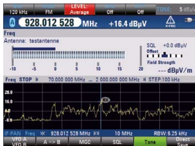
Level measurement of signal at center frequency and its acoustical representation by means of the Tone function.
