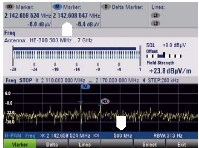
Marker menu selected: 2nd RFI signal IF realtime span of 500 kHz.
