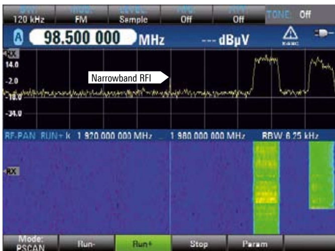
Spectrum and waterfall screen: two mobile phones transmitting in the WCDMA uplink band.
