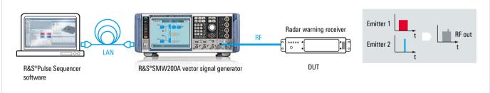
This setup is good for testing a single-channel radar receiver (DUT) in the frequency range up to 40 GHz with 2 GHz signal bandwidth and overlapping pulses (pulse-on-pulse signals). For this application, the R&S\*SMW200A vector signal generator has two integrated baseband generators to generate the pulse-on-pulse signal through internal addition of the baseband signals.
