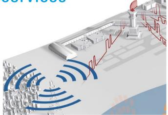
Coexistence testing of radars in the spectral vicinity of base stations or mobile phones requires a mix of communications signals and radar signals. S-band navigation radars operating in the spectral vicinity of LTE base stations or a mobile phone are a typical example. The performance of the radar receiver must be tested against this interference scenario.
