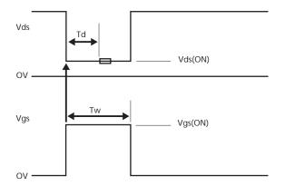
Tds: Drain voltage Vgs: Gate voltage Td: Major delay Tw: Pulse width
