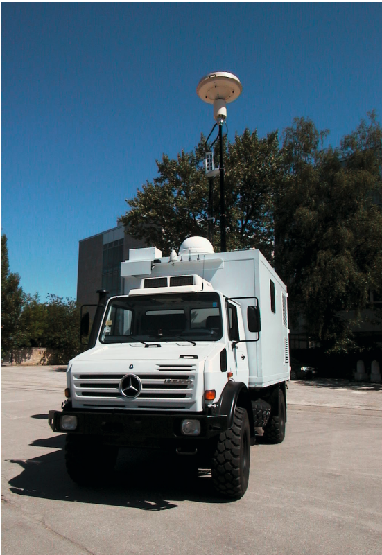
R&S®RAMON radiomonitoring and radiolocation system integrated in a UNIMOG with DF antenna on 6 m mast. Communications via INMARSAT.
