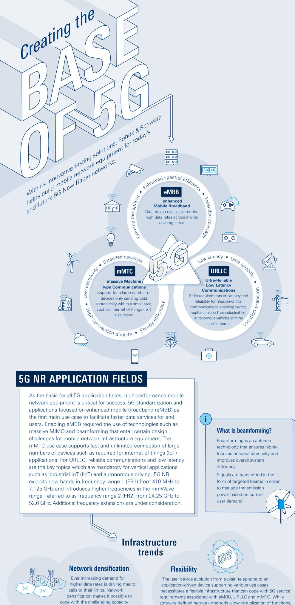
cope with the challenging capacity requirements by complementing macro cells. Depending on the available frequency spectrum and implementation regulations, network densification solutions range from low power small cells to distributed antenna systems (DAS) and mmWave solutions. As one of the first use cases for 5G mmWave applications, last mile fixed wireless
