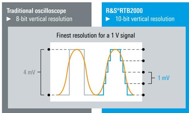
power supplies. The voltages across the switching device must be determined during the on/off times within the same acquisition. For precise measurements of small voltage components, a high resolution of more than 8 bit is essential.
