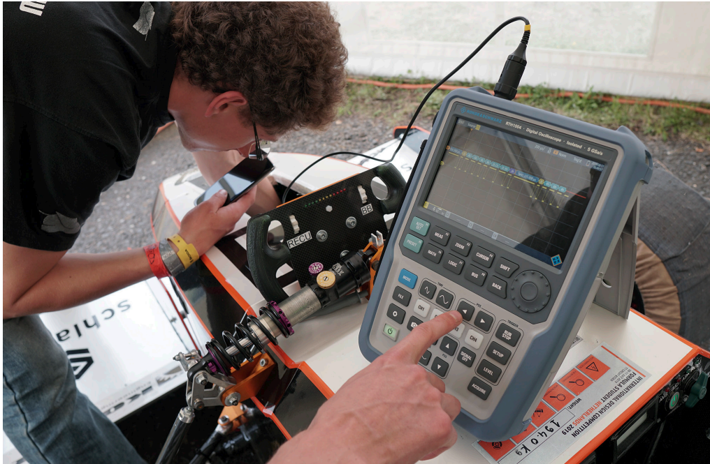
Fig. 4: Debugging at the side of the track using the triggering and decoding option for CAN bus signals. Source: Elephant Racing Team
