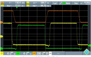
Isolated Inputs for up to 1000 V (RMS) floating voltage measurements eliminates the need for differential high-voltage probes.
