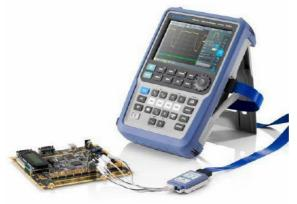
The R&S<sup>®</sup>RTH-B1 mixed signal option allows digital control signals to be captured while analyzing analog input signals.
