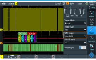
CAN, CAN-FD, LIN and SENT serial protocol trigger & decode with label support for debugging automotive buses.
