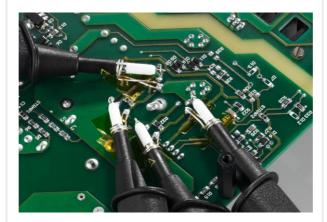
Dedicated 10:1 and 100:1 passive probes allow high-quality floating measurements when connections to the device under test are kept short.
