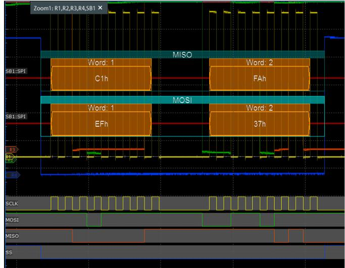
Binary representation of SCLK, MOSI, MISO and SS signals for SPI bus debugging
