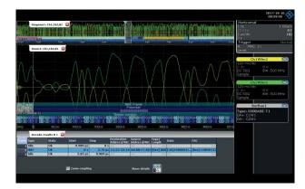
You can debug real-world signals. You see what's happening directly on the bus and isolate specific signals by triggering e.g. on the frame address or on bus errors. Decoding can be shown as a ternary signal, scrambled or descrambled.
