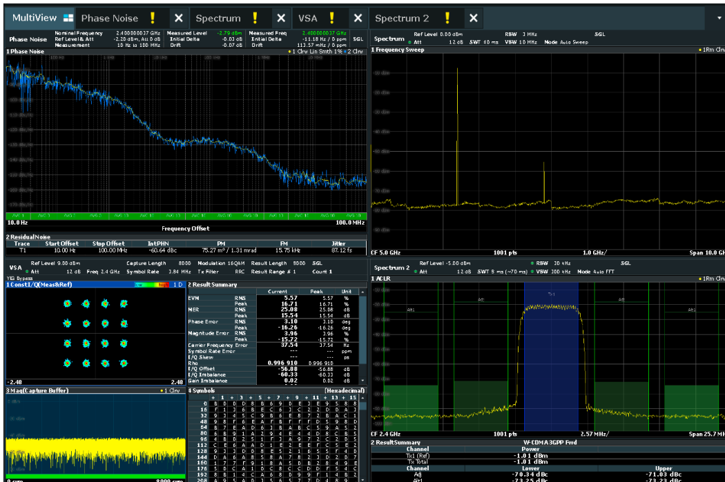
Fig. 6: Signal and spectrum analysis in a single instrument. Right: typical spectral measurements such as adjacent channel power (ACP) or higher-order harmonics. Left (top): phase noise measurement. Left (bottom): vector signal analysis of a digitally modulated signal.
