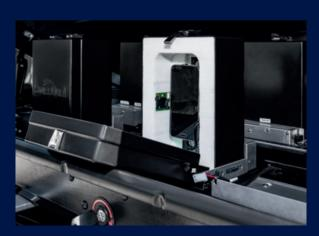
Thermal containment modules ensure uniform and stable conditions for benchmarking campaigns
