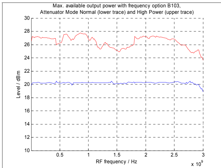
Measured maximum available output level versus frequency
