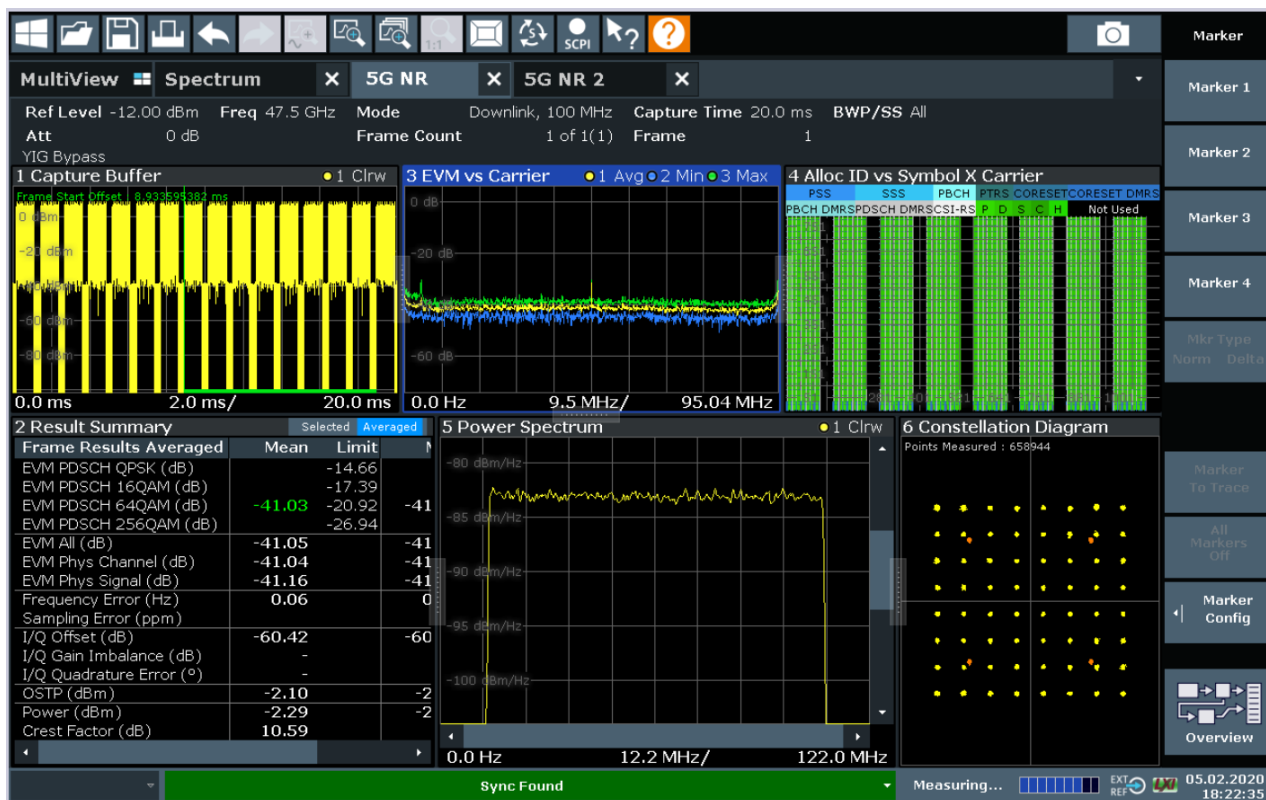
Measured setup error vector magnitude of a 100 MHz wide 5G signal at 47.5 GHz
