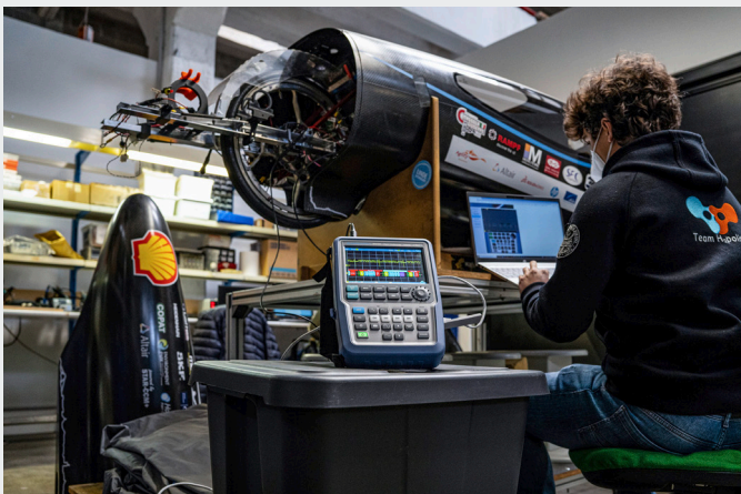
Troubleshooting a CAN in the laboratory.
