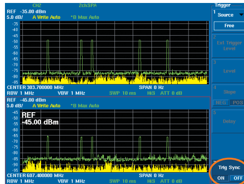
Example of timing measurement of the harmonic burst signal with synchronized sweep
