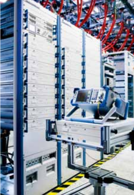
TV transmitter testing with the R&S®ETL.
