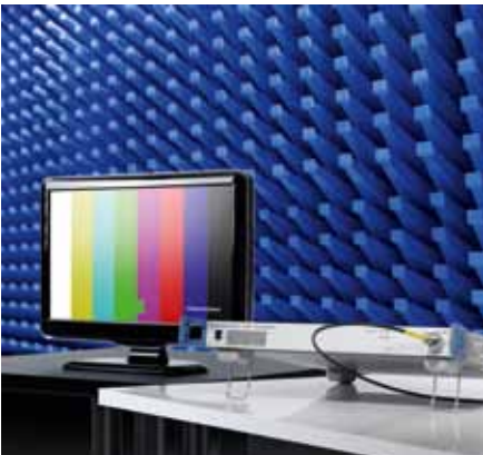
EMC testing of a TV set using the R&S®SFE100.
