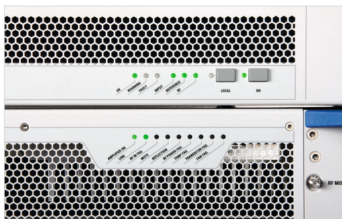
Transmitter status display on the front panel via LEDs.
