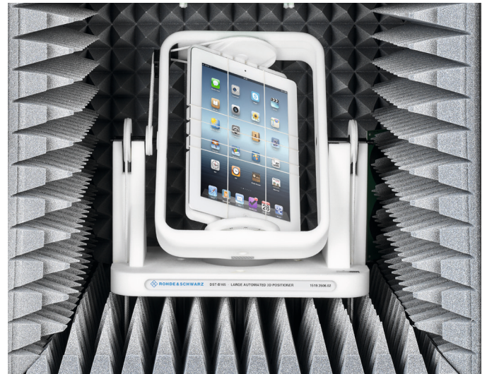
Automated 3D tablet positioner (R&S®DST-B165).
