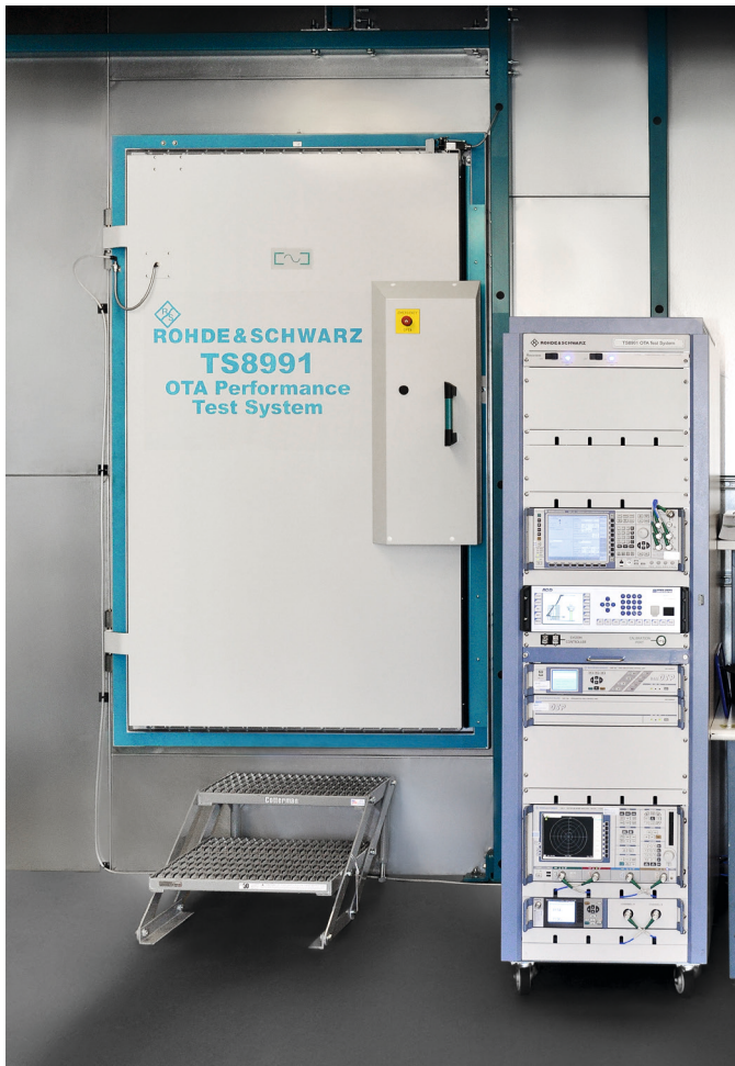
R&S®TS8991 test chamber and system rack (courtesy of 7Layers).
