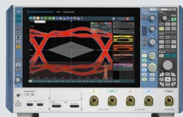
R&S®RTP high-performance oscilloscope for advanced signal integrity analysis
