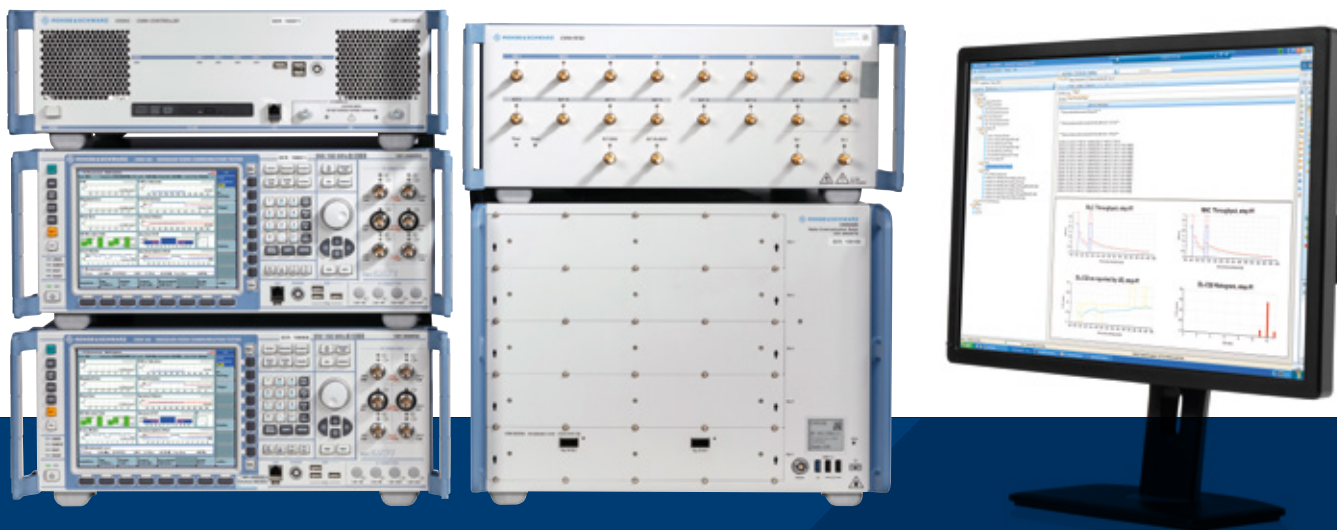
Operator acceptance test setup consisting of two R&S®CMW500, an R&S®CMWC controller, an R&S®CMX500 and the R&S®CMW-RF88 switching matrix.
