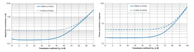
Typical accuracy of transmission magnitude and transmission phase measurements for the R&S<sup>®</sup>ZND; analysis conditions: S<sub>11</sub> = S<sub>22</sub> = 0, cal. power –10 dBm, meas. power –10 dBm, R&S<sup>®</sup>ZND-K5, R&S<sup>®</sup>ZND-K6 or R&S<sup>®</sup>ZND-K8 installed
