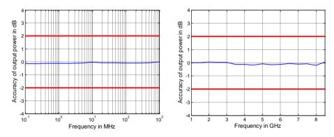
Output power accuracy in dB versus frequency for the R&S<sup>®</sup>ZND base unit
