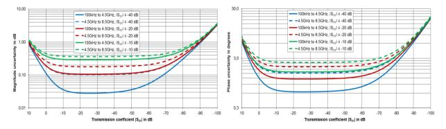
Typical accuracy of transmission magnitude and transmission phase measurements for the R&S<sup>®</sup>ZND; analysis conditions:  $S_{11} = 0$ , cal. power – 10 dBm, meas. power – 10 dBm, base unit or R&S<sup>®</sup>ZND-K1 installed
