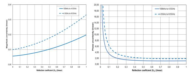
Typical accuracy of reflection magnitude and reflection phase measurements for the R&S<sup>®</sup>ZND; analysis conditions: S<sub>12</sub> = S<sub>21</sub> = 0, cal. power –10 dBm, meas. power –10 dBm, R&S<sup>®</sup>ZND-K5, R&S<sup>®</sup>ZND-K6 or R&S<sup>®</sup>ZND-K8 installed
