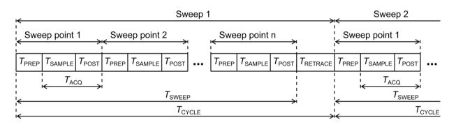
$T_{PREP}$  Preparation time required to set up the internal hardware components
