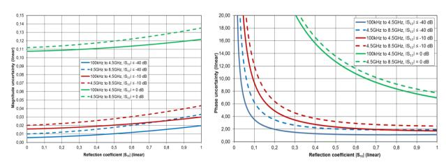
The accuracy of reflection measurements is reduced for non-isolating DUTs, i.e.  $|S_{12}| > 0$  using a unidirectional test set.
