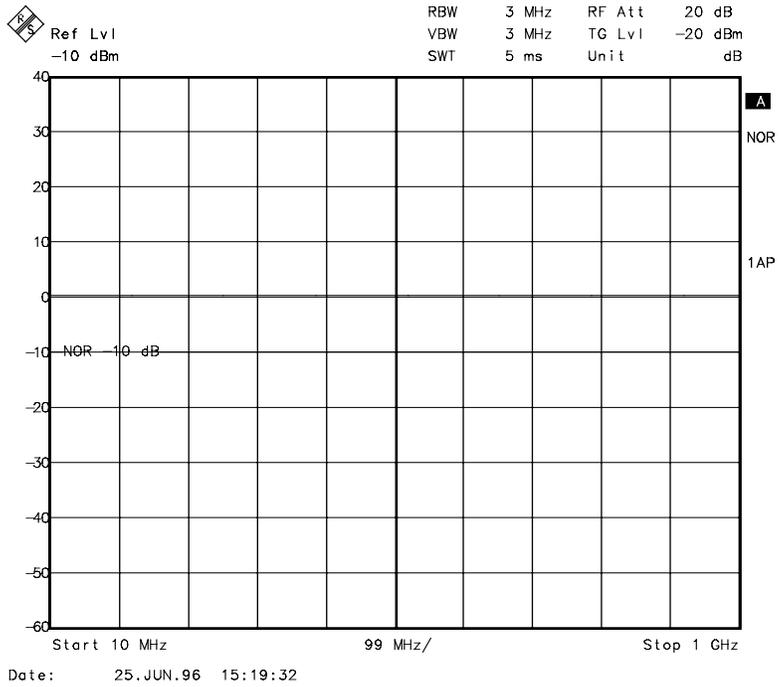
Fig. 2.13-5 Measurement with REF VALUE 20 dB and REF VALUE POSITION 50%
