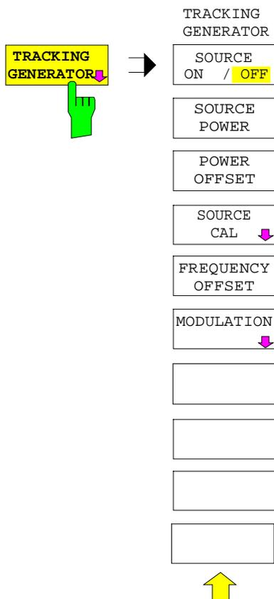
The *TRACKING GEN* softkey opens a menu for setting the functions of the tracking generator.
