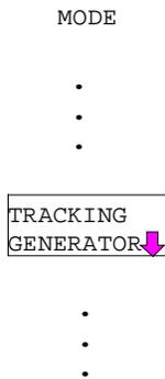
The *MODE* key activates the menu in which the submenu for setting the tracking generator can be selected in addition to different operating modes.
