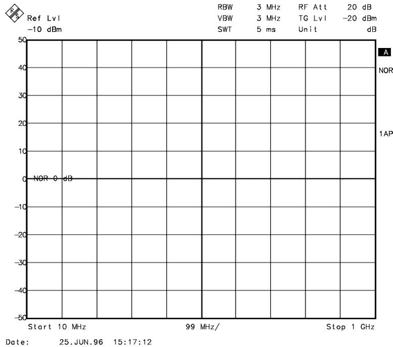
Fig. 2.13-4 Normalized measurement, shifted with *REF POSITION* 50 %
