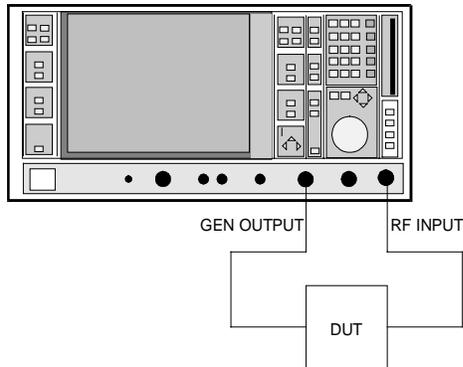
Fig. 2.13-1 Test setup for reflection measurements
