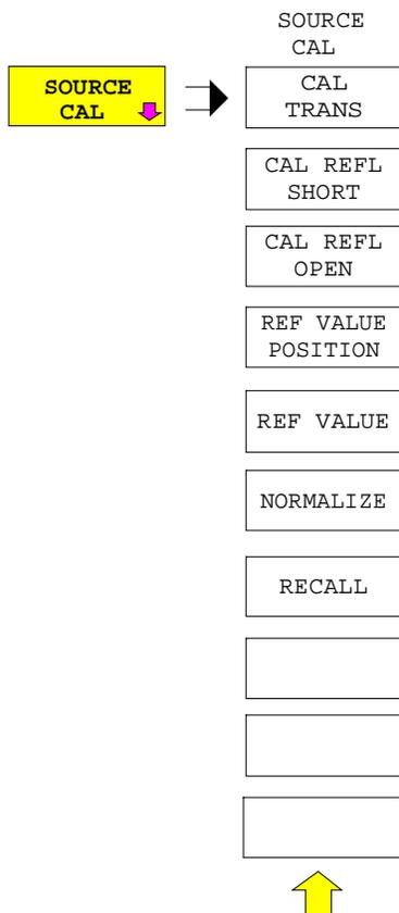
The *SOURCE CAL* softkey opens a submenu comprising the calibration functions for the transmission and reflection measurement.
