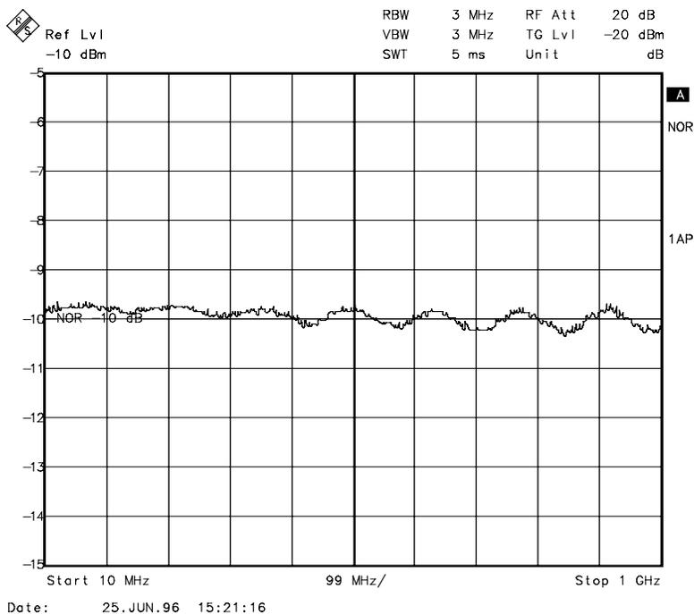
Fig. 2.13-1 Measurement of a 10dB attenuator pad with 1 dB / Div
