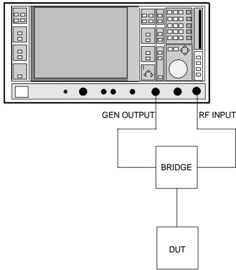
Fig. 2.13-6 Test setup for reflection measurements
