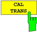
The *CAL TRANS* softkey triggers the calibration of the transmission measurement.
