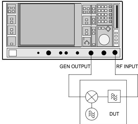
Fig. 2.13-7 Test setup for frequency-converting measurements
