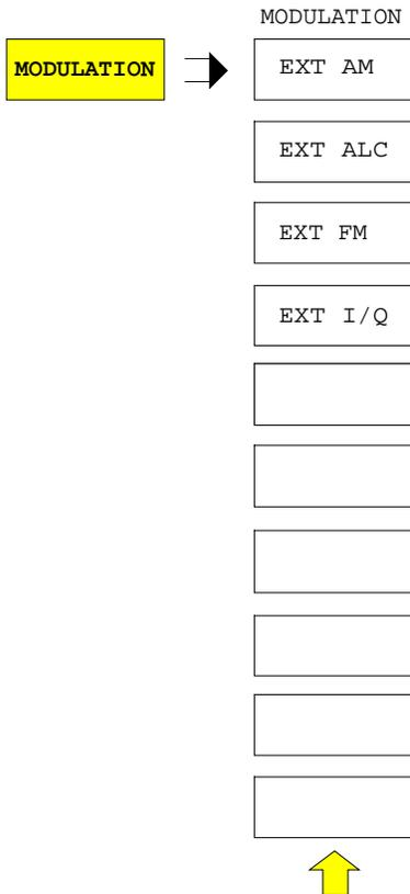
The *MODULATION* softkey opens a submenu for selecting the different modulation types.
