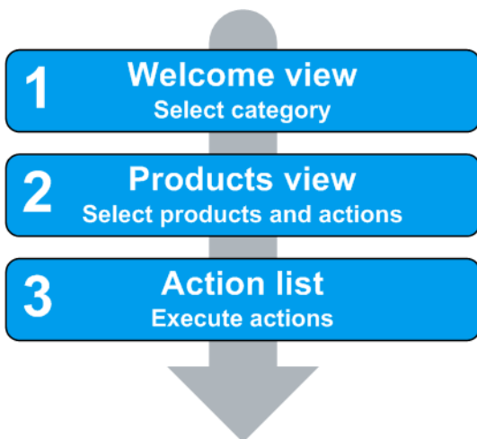
Figure 2-3: Three-step software update procedure
