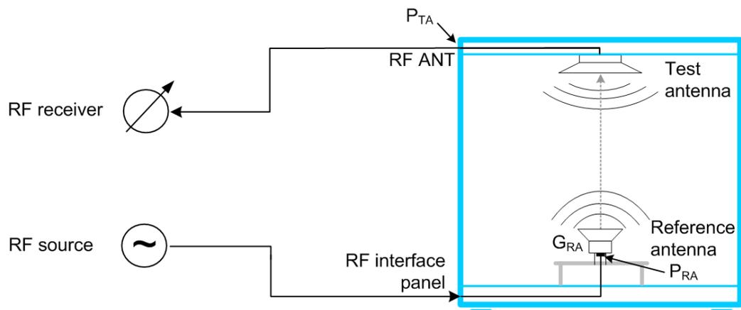
**Fig. 1-1: Schematic test setup for reference path loss measurement**
