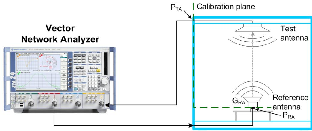
Fig. 1-3: VNA test setup for transmission measurement
