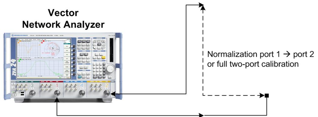
Fig. 1-2: VNA test setup for cable calibration
