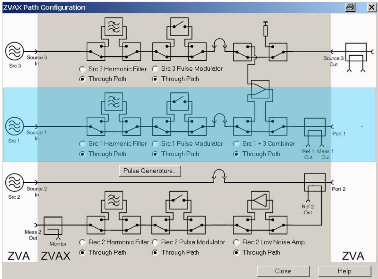
**Fig. 1-2: ZVAX Path Configuration**
