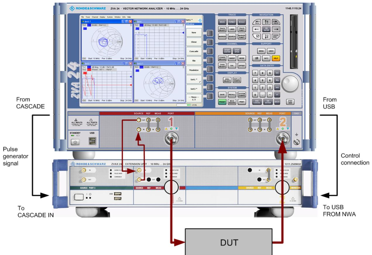
Fig. 1-1: Test setup for pulse profile measurement
