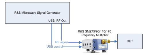
This example explains the starting up with a multiplier without attenuator. You can also find tips on how to proceed if you are using an R&S SMZ with an attenuator.
