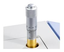
R&S SMZ instruments with mechanical level control are equipped with a power adjustment screw on top.
