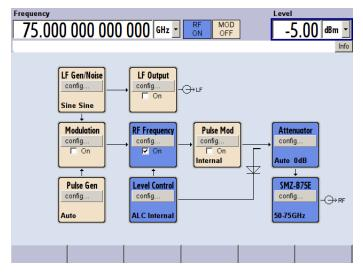
Figure 6-4: Block diagram of the R&S SMF indicating a connected R&S SMZ with electronic level control
