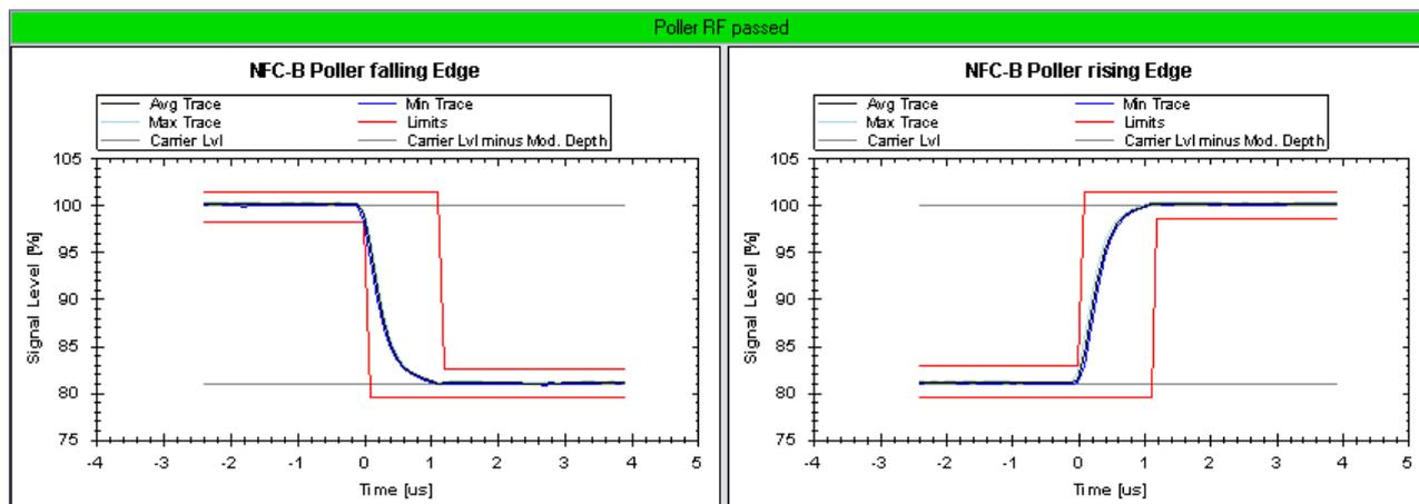
**Fig. 3-4: NFC-B poller signal (based on example file NFC-B\_Example.iq.tar); NFC-F looks similar**
