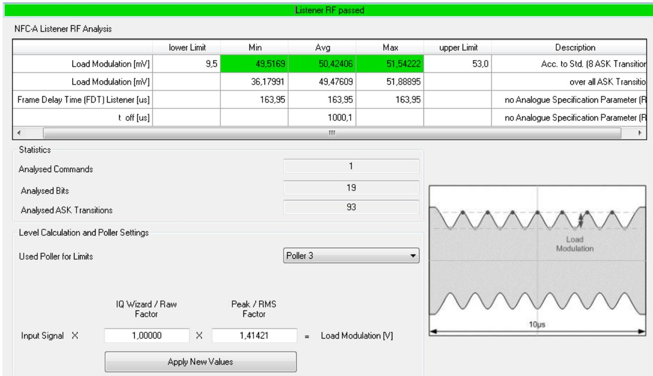
**Fig. 3-15: Listener results of an NFC-A signal (based on example file NFC-A\_Example.iq.tar)**
