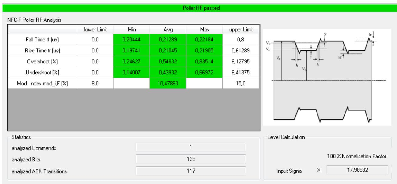
**Fig. 3-12: Poller results of an NFC-F signal (based on example file NFC-F\_424kB\_Example.iq.tar)**
