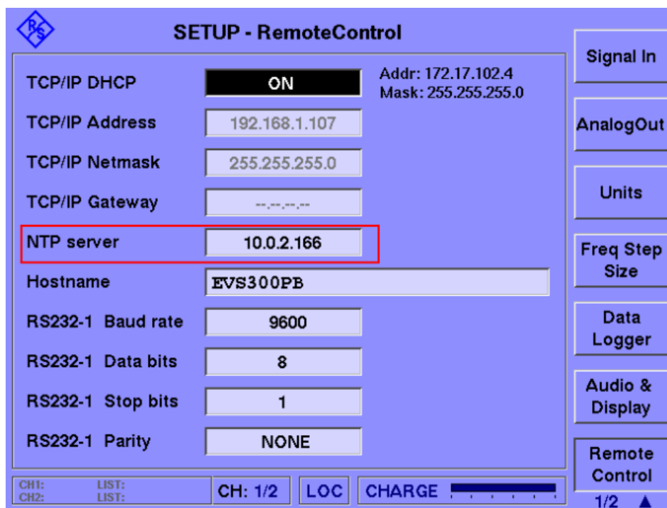
Fig. 5-3: NTP Server configuration
