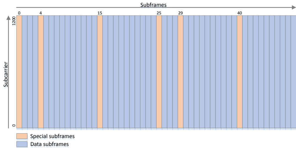
Figure 4-1: Radio frame as defined by the V5GTF standard
