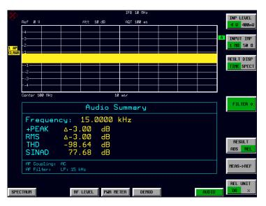
Fig.2-15 Audio measurement in relative mode
