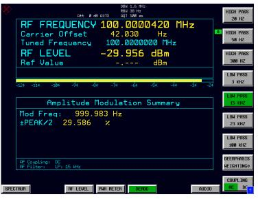
Fig.2-10 AM Modulation measurement in the DEMOD mode
