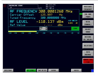
Fig.2-8 Tuned RF Level measurement with Averaging
