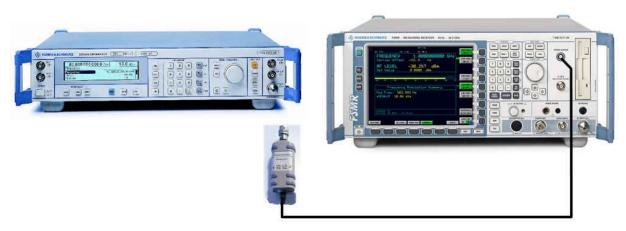
Fig.2-2 RF Power measurement setup
