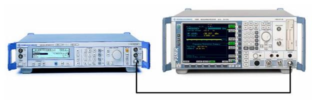
Fig.2-9 AM modulation measurement setup
