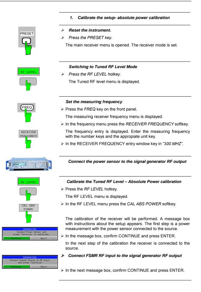
The FSMR is now calibrated in one RF level range (the upper level range does handle RF levels from -10 dBm to +30 dBm). Measurements in this level range can now performed with full accuracy.
