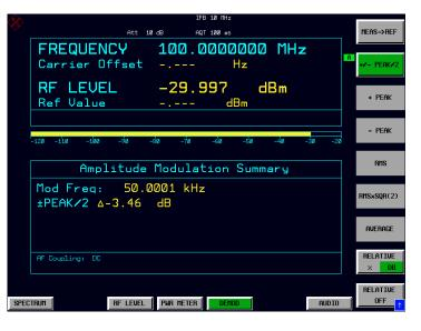
Fig.2-11 Relative measurement in the demod mode
