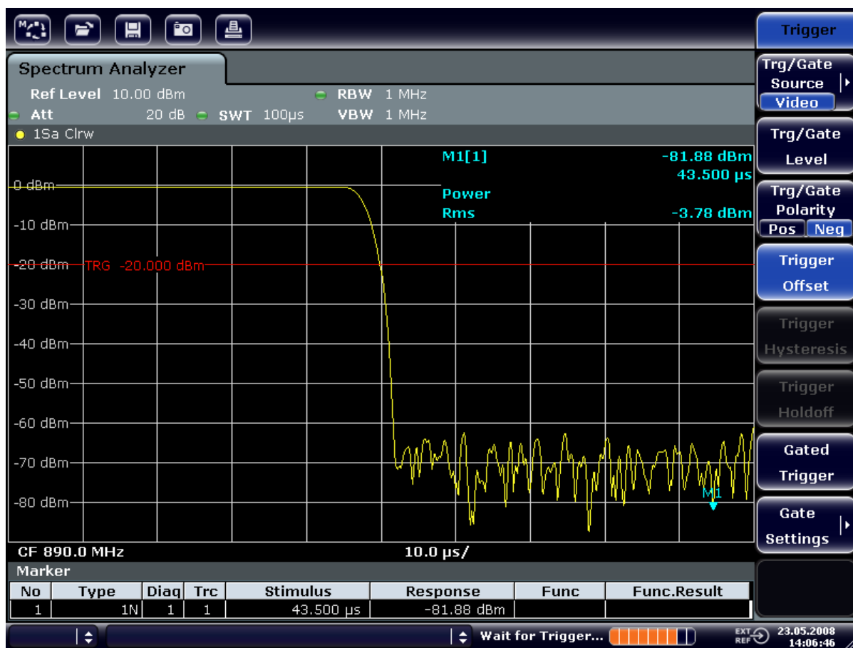
Figure 7-10: Falling edge of the GSM burst displayed with high time resolution
