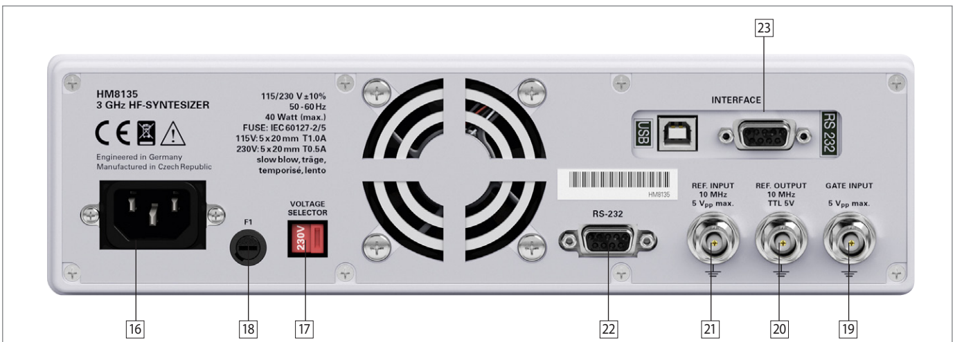
Fig. 2.2: Rear panel of the HM8135
