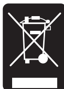
Fig. 1.4: Product labeling in accordance with EN 50419
