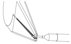
Use pliers to grip and pull the probe tip carefully out of its contact socket.
