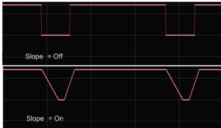
Figure 4-2: Impact of the "Slope" parameter ("RLC Curve" = Off)
