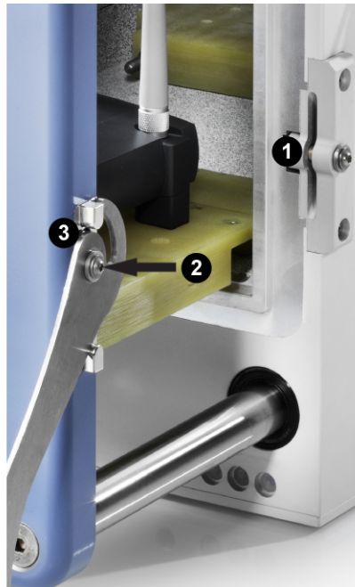
Figure 6-1: Additional points for greasing (manual version)
