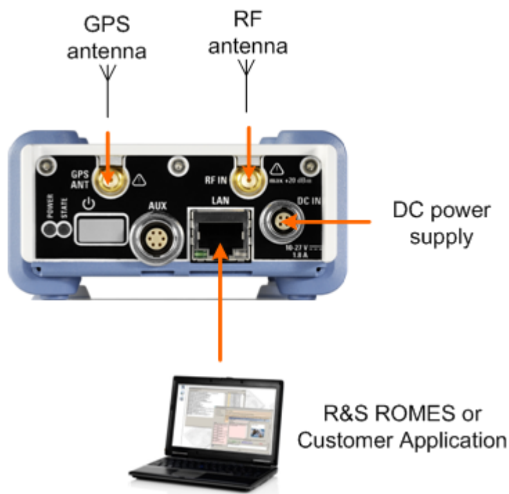
Figure 1-1: Typical measurement setup with the R&S TSME
