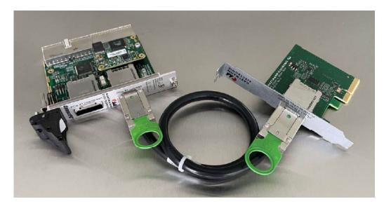
Figure 3-10: Cabling of the R&S TS-PSC08 components.
