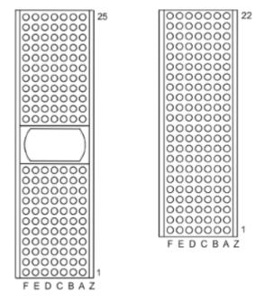
Figure 5-4: Connectors P1 and P20 rear (mating side)
