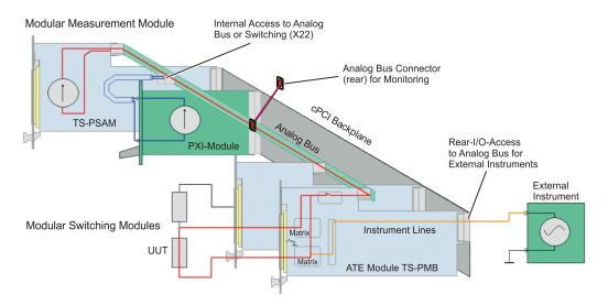
Figure 4-9: Use of the analog bus in the R&S CompactTSVP (example)
