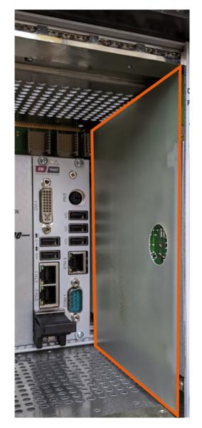
Figure 3-7: Install insulation plate
