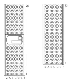
Figure 5-2: Connectors P1 and P20 front (mating side)
