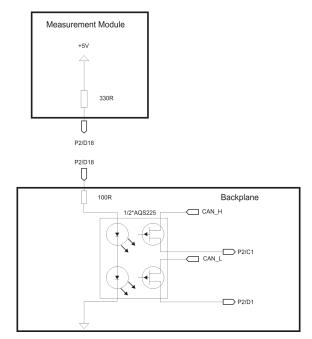
Figure 4-5: Wiring CAN bus
