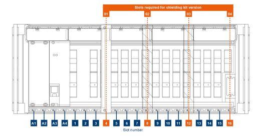
Figure 3-3: Slot requirement for installation of shielding kit
