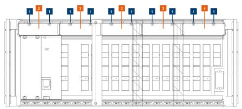
Figure 3-4: Mount shielding kit covers (front view)
