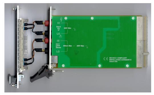
Figure 4-11: Adaption of a short PXI module to the adapter interface (example)
