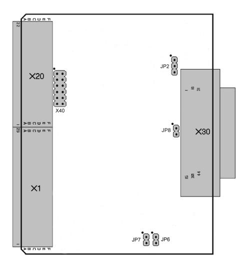
Figure 4-16: Connectors and Jumpers on the R&S TS-PSYS1 1152.4004.02
