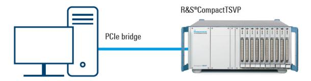
Figure 3-9: R&S CompactTSVP to external PC connection
