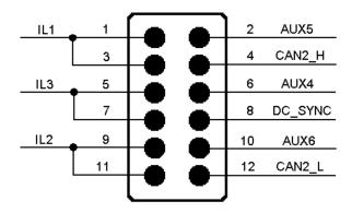
Figure 5-25: Signals at the R&S TS-PSYS1 jumper field X40
