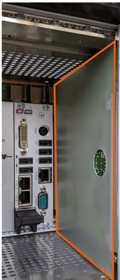
Figure 3-7: Install insulation plate
