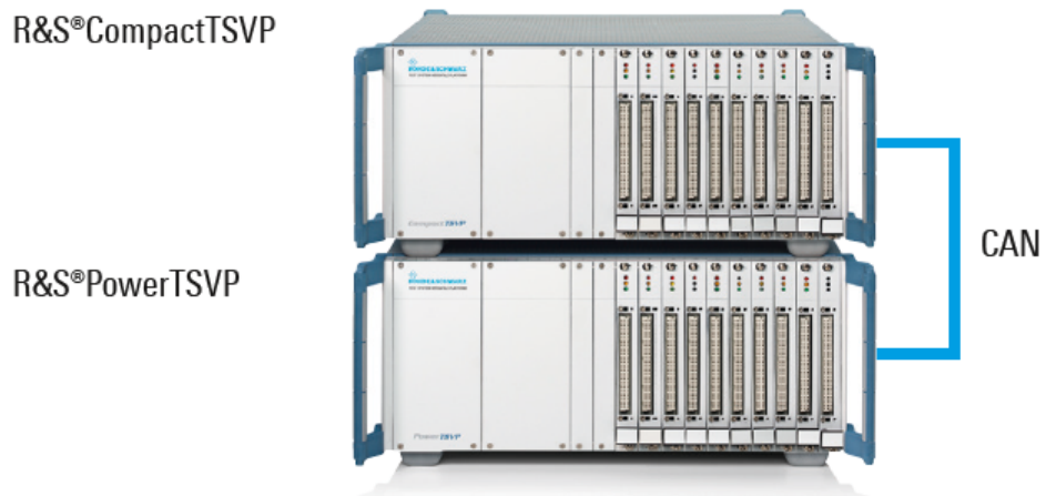
Figure 3-8: R&S CompactTSVP to R&S PowerTSVP connection
