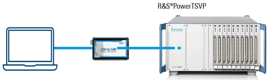
Figure 3-11: R&S PowerTSVP to external PC connection
