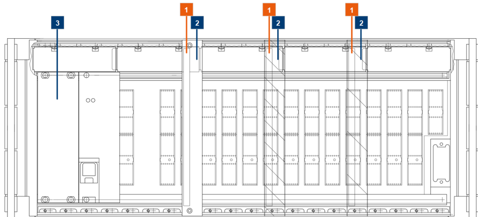
Figure 3-6: Finish shielding kit installation
