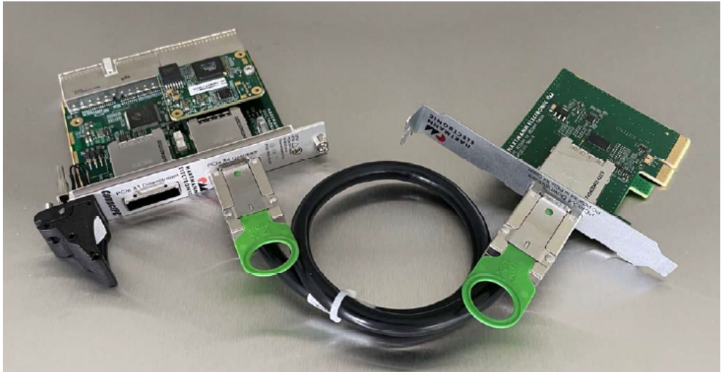
Figure 3-10: Cabling of the R&S TS-PSC08 components.
