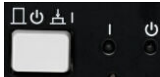
Figure 2-5: Standby switch and LEDs
