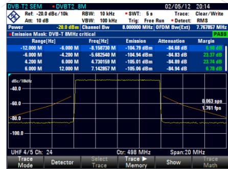
2nd step: Measuring the spectrum emissions in front of the transmitter output filter using a directional coupler and applying the output filter transducer data
