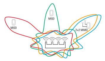
Fig. 3: Multi-user MIMO system with spatial multiplexing based on beamforming
