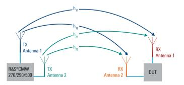
Fig. 1: In spatial multiplexing, each receive antenna receives a sum signal consisting of all of the transmitted signals. The prevailing channel conditions are represented in a transmission matrix H with elements  $h_{mm}$ .
