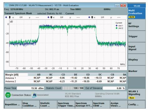
Fig. 4: The transmit spectrum mask measurement determines the power distribution with respect to the total transmit power for both MIMO transmitters within a frequency range. It is easy to identify unwanted signals outside the permissible frequency range.
