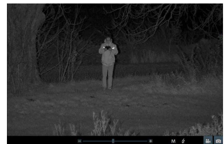
Fig. 2: One advantage of using radiomonitoring is the ability to locate the remote control and the drone pilot. R&S®ARDRONIS cameras use infrared optics to allow the drone pilot to be uncovered even at night.
