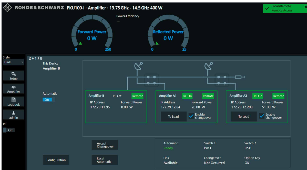
Fig. 4: Three R&S®PKU100 uplink amplifiers, configured as a 2+1 system, are managed by the integrated system control function. If an active amplifier fails, the backup unit takes over in a fraction of a second.
